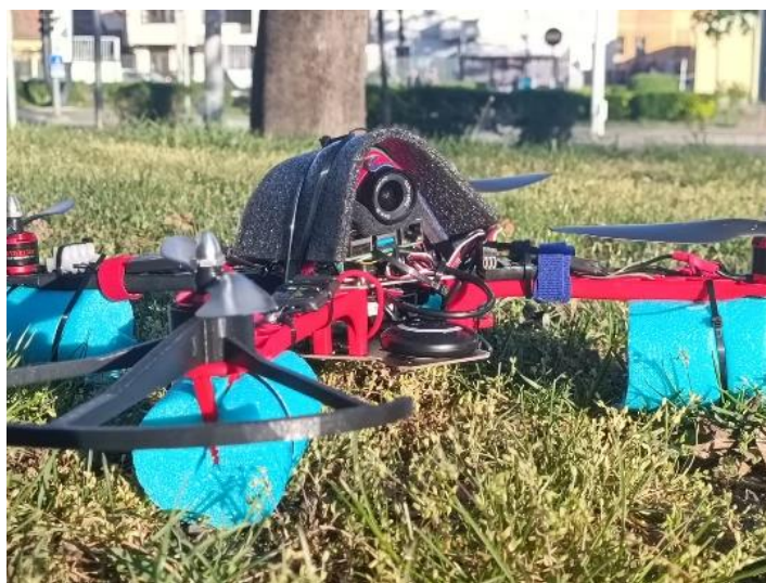
Figure 1. Designed UAV platform with video streaming capabilities
